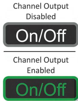
Enable or disable the output of the selected channel. To select a channel, refer to Channel Selection.
