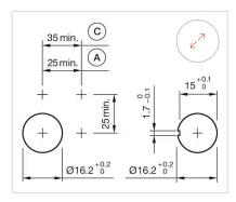
$\label{eq:Absolute} \begin{array}{l} A = Solder/Plug-in \ terminal \ 2.8 \ mm \ x \ 0.5 \ mm \\ C = Screw \ terminal \end{array}$
