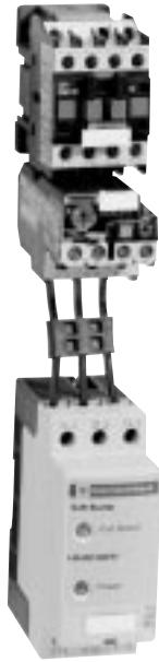
LH4N soft starts provide gradual, smooth starting of single phase and three phase squirrel cage motors. Its modular design is intended for use downstream of an electromechanical start for reduction of the mechanical jolts, which may occur when started across the line.
