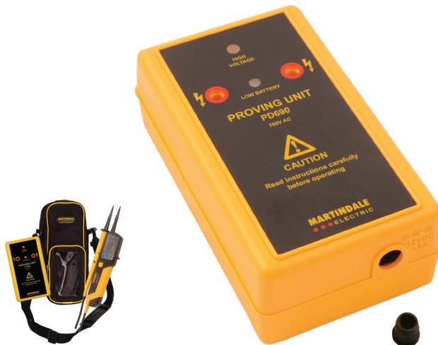
The PD690 proving device produces 700V AC/DC to enable voltage indicators and other devices with ranges up to 700V to be checked. It is a portable, battery powered proving unit with the option of being driven from a 12V supply via a car or mains power supply. The kit is supplied with a combination carry case for both VI and PD products.
