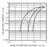
Fig.3 Grounded emitter propagation characteristics
