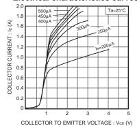
Fig.1 Groundede emitter output characteristics ( I )
