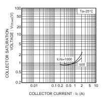
Fig.6 Collector-emitter saturation voltage vs. collector current
