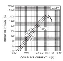
Fig.5 DC current gain vs. collector current ( II )
