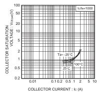
Fig.7 Collector-emitter saturation voltage vs. collector current
