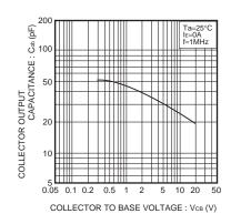
Fig.8 Collector output capacitance vs. collector-base voltage
