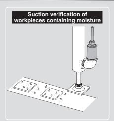
Note: When vacuum is released, take precautions to avoid water collision with inertia force. (An adapter with restrictor (ZS-31-X175) is available to prevent water collision with rush inertia.) (Refer to "NOTE" on the Operation Manual at SMC website for details.)
