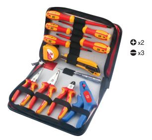
This set of insulated RS PRO precision tools is supplied in a VDE approved vinyl wallet for secure transport and storage and features a wide variety of tools to be able to complete most applications, especially when working with live electrics or energised circuits. The cutters, pliers and screwdrivers are ideal for working up to 1000 V AC or 1500 V DC, making them essential tools for safe working in a professional or home DIY capacity.
