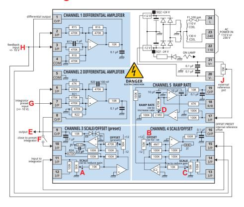
**Options:** If the system is unstable and slowly oscillates, try adding another 1 μF at the **J1** position (CHANNEL 3). The bipolar capacitor sets the integrator time constant.
