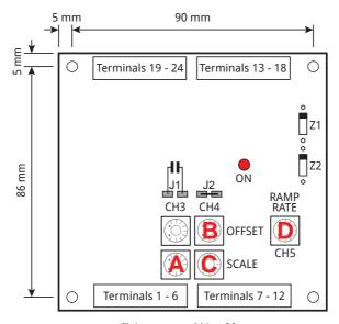
Fixing screws: M4 x 20 mm
