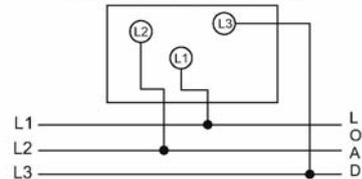
**AC Voltmeters 3 Phase 4 Wire**
