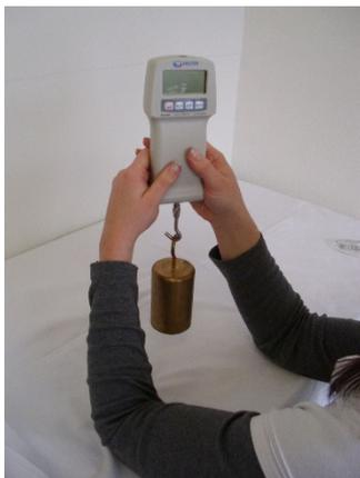
5. Hold position until “**F**” appears on the display. In this case remove weight and adjustment is completed. In case of “**E**” is displayed - repeat step 1. to 5. until “**F**” attests a successful adjustment.
