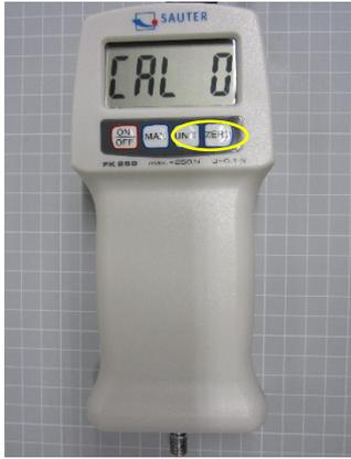
3. Wait a few seconds and display will show the necessary **adjustment weight**, e.g. 5,000kg for FK 50 or 10,00kg for FK 100.
