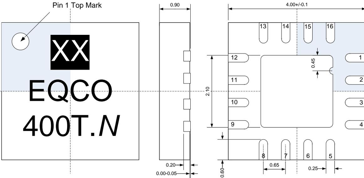
Figure 6: Package Drawing viewed from Top - Side - Bottom<sup>4</sup>
