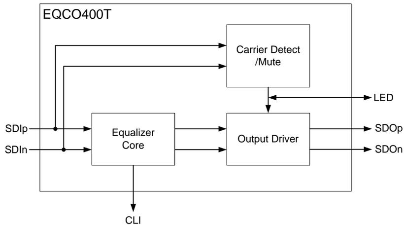
Figure 2: EQCO400T8 block diagram showing electrical connections
