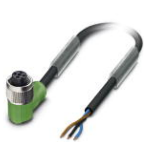
Sensor/Actuator cable, 3-position, PUR halogen-free, Black-gray RAL 7021, Free cable end, on Socket angled M12, A-coded, Cable length: 10 m
