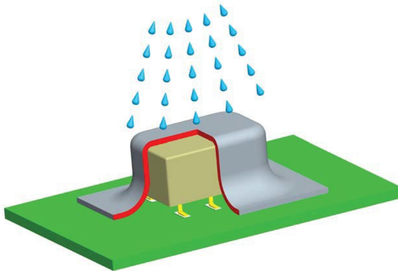
Fig. 4: Coating of relays on PCB's
