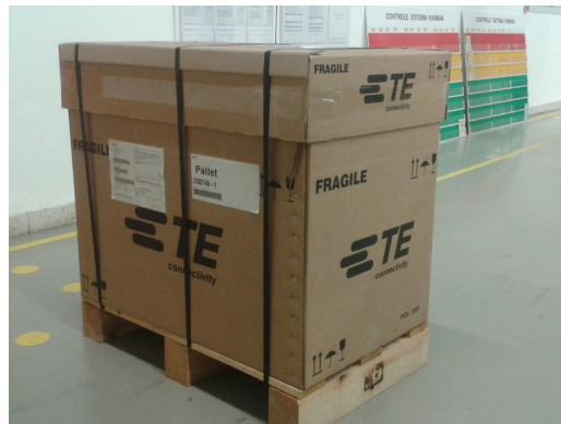
Fig. 1: Proper packing of relays for transportation
