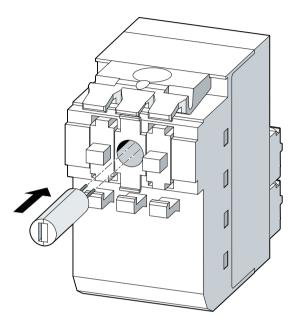
Mount the integrated illumination LED on the rear face of the interface module.
