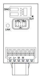
One spring-loaded or screw terminal (6-pole) is available for connecting the supply cables:
