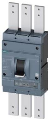
circuit breaker 3VA2 IEC Frame 1250 breaking capacity class M  $I_{cu}=55\text{ kA}$  @ 415 V 3-pole line protection ETU330 LIG  $I_{n}=1250\text{ A}$  overload protection  $I_{r}=500\text{ A}$  ...1250 A short-circuit protection  $I_{i}=15\ldots10 \times I_n$  ground-fault protection  $I_{g}=02\ldots1 \times I_n$   $t_g=01/03\text{s}$  circuit breaker with straight bus connectors extended
