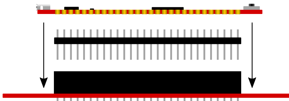
Figure 2-1. Attaching Pin-Headers to the Curiosity Nano Board
