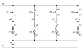
E1: circuit-breaker ON E2: circuit-breaker OFF
