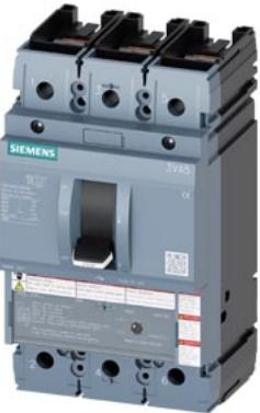
circuit breaker 3VA5 UL Frame 250 breaking capacity class H 65 kA @ 480 V 3-pole, line protection TM210, FTFM,  $In=30$  A overload protection  $Ir=30$  A permanently set short-circuit protection  $li=11.67 \times In$  UL 489 SB (naval), 50 °C, cable connection on two sides
