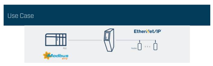
The Anybus Communicator EtherNet/IP scanner to Modbus RTU server enables you to connect any EtherNet/IP device to Modbus RTU control systems.
