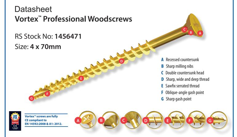
The recessed double countersunk head on the Vortex<sup>™</sup> product range reduces the likelihood of shearing the head of the screw, whilst assisting the completion of countersinking, making it a more reliable product for users.
