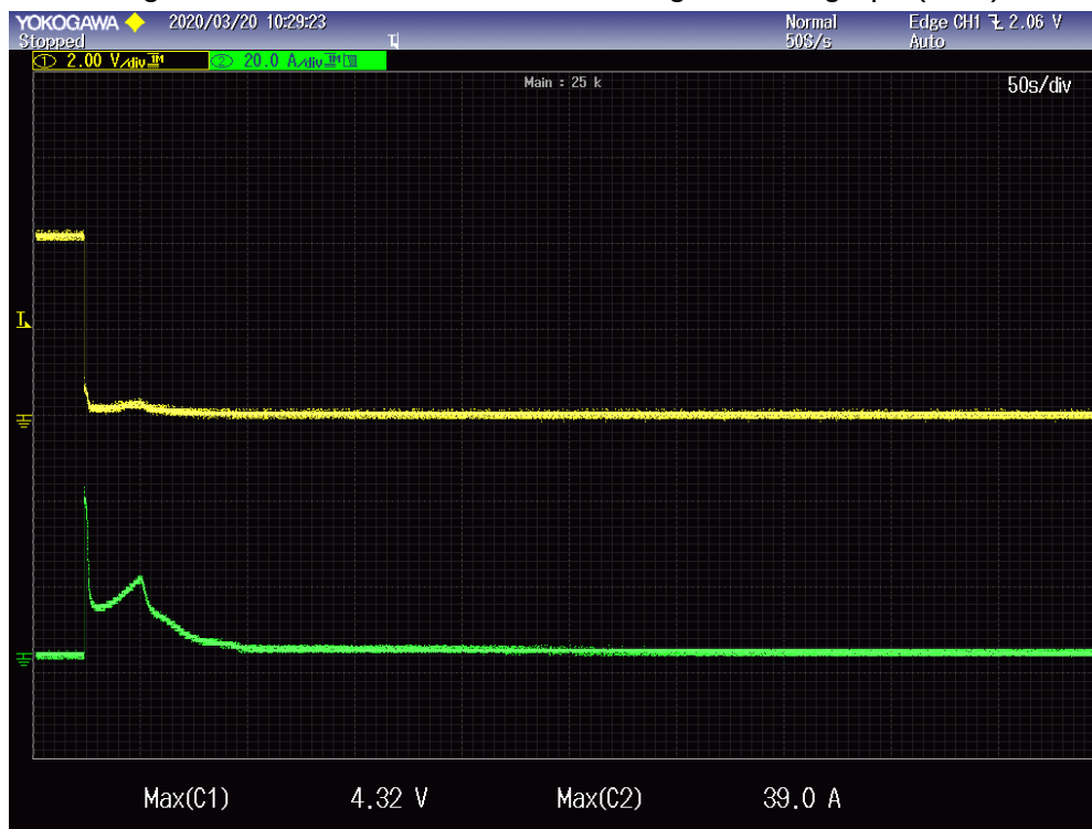
Figure 38: External short circuit – voltage/current graph (cells)
