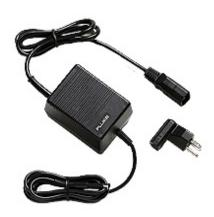
Provides power cord operation and charging for Fluke 430 Series Power Quality Analyzers Mains (Line Voltage): switchable 115 V  $\pm$  15% or 230 V  $\pm$  15% Equipped with a male receptacle plug that must be connected to a line cord/adapter appropriate for local use. (Line cord/adapter not included)
