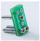
The Tag-Connect Clip Board attaches to the alignment pins of a Tag-Connect No Legs cable such as TC2030-MCP-NL. The Clip Board can be pressed onto the alignment pins from underneath the circuit board, providing a temporary connection for debugging purposes. Then you have the best of both worlds: a small PCB footprint and a reliable debugging connection. Note: Clip Boards are small and easily misplaced, so we include 3 in the package.
