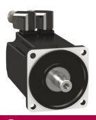
servo motor BMH - 3.3 Nm - 6000 rpm - untapped shaft - with brake - IP54
