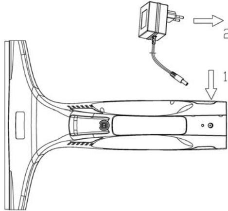
**Note:** during the charging process, the charge indicator is red, once the battery is fully charged it will turn blue.
