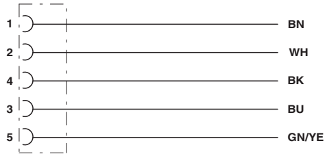
Contact assignment of the M12 sockets
