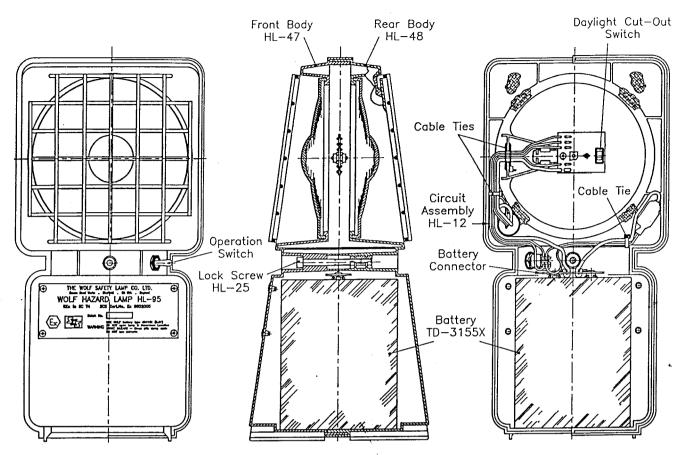
The Wolf Hazard Lamp HL-95 has recently been certified to the European EN50 Standards concerning Electrical apparatus for potentially explosive atmospheres. It is one of the first products to carry a 1995 "D" certificate, issued by Sira Certification Service. Testing to Factory Mutual requirements, as recognised in the USA, is expected to be completed within a matter of months.
