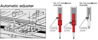
Automatic adjusters are used widely throughout industry to boost efficiency and reduce the costs of adjustment work. Vessel makes a wide range of products as attachments for automatic adjuster. Before mounting, check the jig outer diameter and total length. Use the above installation example as reference.
