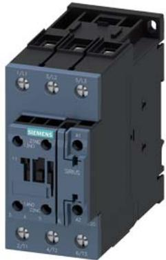
traction contactor, AC-3e/AC-3, 80 A, 37 kW / 400 V, 3-pole, 110 V DC, 0.7-1.25\* Uc, solid-state operating mechanism, with integrated varistor, auxiliary contacts: 1 NO + 1 NC, screw terminal, frame size: S2
