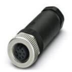
Connector, 8-position, Socket straight M12, A-coded, Screw connection, Knurl material: Zinc die-cast, nickel-plated, Cable gland Pg11, External cable diameter 8 mm ... 10 mm
