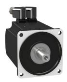
servo motor BMH, Lexium 32, 10.3Nm, 4000rpm, keyed shaft, with brake, IP54, 16 multiturn encoder
