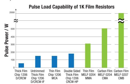
Thin Film MELF resistors are frequently used in applications that experience high-pulse loads:
