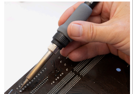
T18-SB Shape-SB Narrow-pitch Soldering Type (Shape S)
