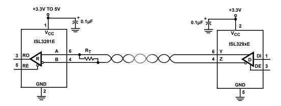
FIGURE 1. NETWORK WITH ENABLES
