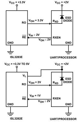
FIGURE 6. USING V<sub>L</sub> PIN TO ADJUST LOGIC LEVELS
