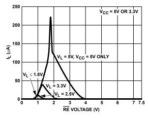
FIGURE 8. V<sub>L</sub> SUPPLY CURRENT vs ENABLE PIN VOLTAGE
