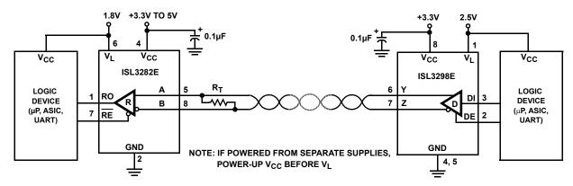
FIGURE 3. NETWORK WITH  $V_{L}$  PIN FOR INTERFACE TO LOWER VOLTAGE LOGIC DEVICES
