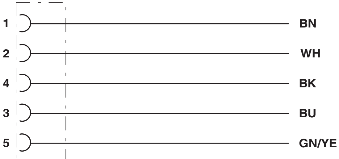
Contact assignment of the M12 sockets
