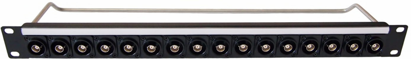
RS30184 - 1U Rack loaded with 16 x 50 Ohm Insulated BNC. M3 Holes. Front mounted
