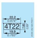
MAR.12 - Marker label for devices with DIP switches
