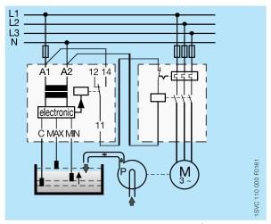
Liquid level control - fill - selected function "T" (UP)
