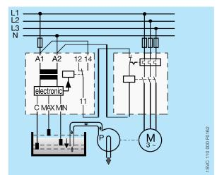
Liquid level control - drain - selected function " $\downarrow$ " (DOWN)
