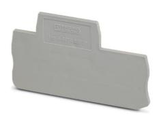
End cover, Length: 71.5 mm, Width: 2.2 mm, Height: 47.5 mm,
