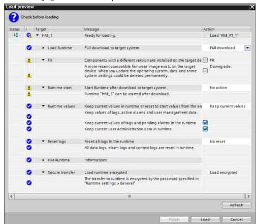
If the connection was established successfully, the "Load preview" dialog box is displayed. The following figure shows an example.
