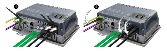
Next, use cable ties to secure the cables to the marked fastening points.
