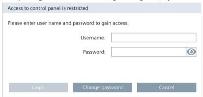
Enter the desired login name with the associated password and log in using the "Login" button.
