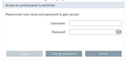
Log in as a user with the "Control Panel access" function right to activate the password protection for the Control Panel. Use the following button to make the password visible for the display duration of the dialog:
