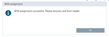
13. Remove the RFID card from the reader and select "OK".
