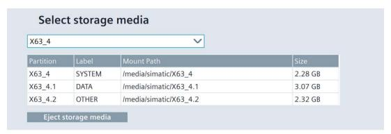
The drop-down list box shows all the storage media at the interfaces of the HMI device.
