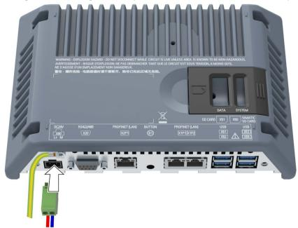
4. Verify the correct polarity of the cables using the interface labeling on the back of the HMI device.
