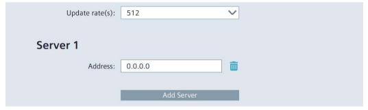
From the "Update rate(s)" list, select the desired synchronization interval, ranging from 8 to 65536 seconds (approx. 18 hours). Default setting: 512
