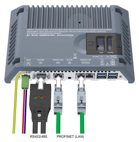
Use the PROFINET (LAN) X1 or X2 interface for SIMATIC process connection. Use the RS 422/485 interface for controllers from other manufacturers that are connected at the serial interface. Additional information on compatible controllers is available in the section "Communication with controllers (Page 195)".
