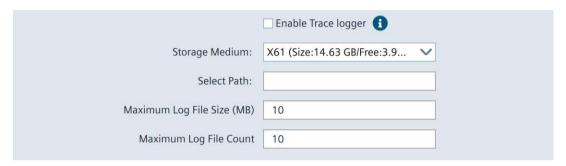
• "Enable Trace logger": Option to back up "tracing" information on an external storage medium. The default setting is "deactivated".
