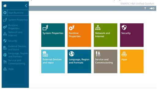
2. If desired, operate the project or configure the HMI device via the Control Panel. If you no longer need the HMI device, switch it off.
