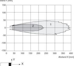
Curve1:flat surface 100mm×100mm Curve2:round bar, Ф25mm
