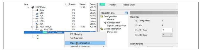
The address of the ASi slave is then set in the device configuration on the master under "Station table".
