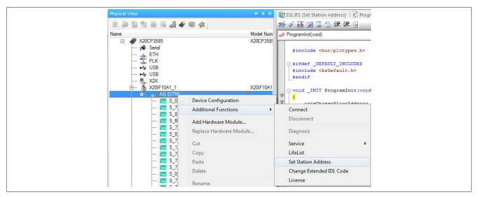
First, the slave to be addressed is selected and the desired new address is specified. A new address can be assigned using "Set address".
