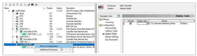
• Confirm and save all settings with OK. The configuration is transferred to the controller and, if correct, a connection between master and slave is automatically established.
