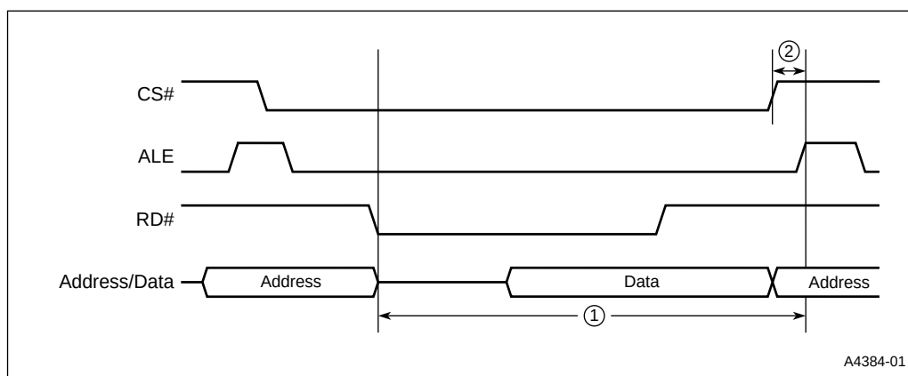
Figure 1. Bus Cycle for Mode 0 or Mode 1 Operation (Read Cycle)
