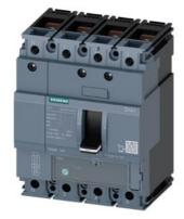
circuit breaker 3VA1 IEC frame 160 breaking capacity class N Icu=25kA @ 415V 4-pole, line protection TM220, ATFM, In=40A overload protection Ir=28A...40A short-circuit protection Ii=10 x In N conductor unprotected nut keeper kit
