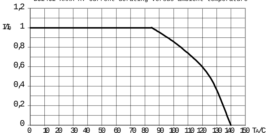
B82462-XXXX-X: current derating versus ambient temperature
