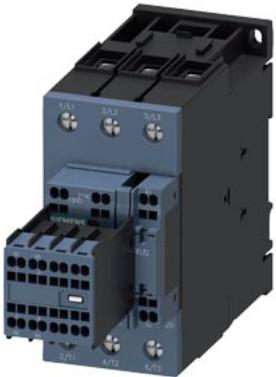
power contactor, AC-3e/AC-3, 65 A, 30 kW / 400 V, 3-pole, 48-80 V AC/DC, 50/60 Hz, with integrated varistor, auxiliary contacts: 2 NO + 2 NC, main circuit: screw terminal, control and auxiliary circuit: spring-loaded terminal, size: S2, removable auxiliary switch
