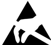
When returning modules, assemblies or components, the regulations of EN 100 015 "Protection of electrostatically sensitive components" must be observed. Use only the appropriate **ESD** packaging for transport.
