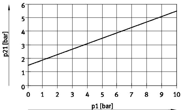
Minimum pilot pressure p_{21} as a function of operating pressure p_1
