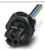
PRC device connector, black, 3-pos., 6 mm²/630 V/35 A, crimp connection, with 150 mm cable length, cut flat at the end
