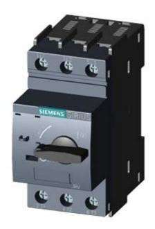
CIRCUIT-BREAKER SZ S00, RATED CURRENT 1.25A, N-RELEASE 16A, FOR STARTER COMBINATION, SCREW CONNECTION, STANDARD SW. CAPACITY
