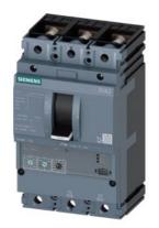
circuit breaker 3VA2 IEC frame 160 breaking capacity class M lcu=55kA @ 415V 3-pole, motor protection ETU350M, LSI, In=100A overload protection Ir=40A...100A short-circuit protection Isd=3...15 x Ir, Ii=15 x In nut keeper kit
